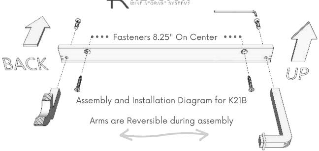
Includes screws and wrench to assemble the arms as well as 1" wood screws to secure the Kessick Wine Hardware a wood surface.
