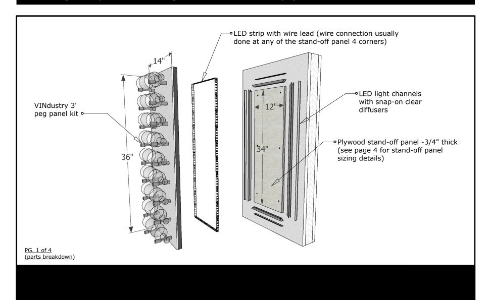
Rectangular panel LED light and stand-off plywood installation
