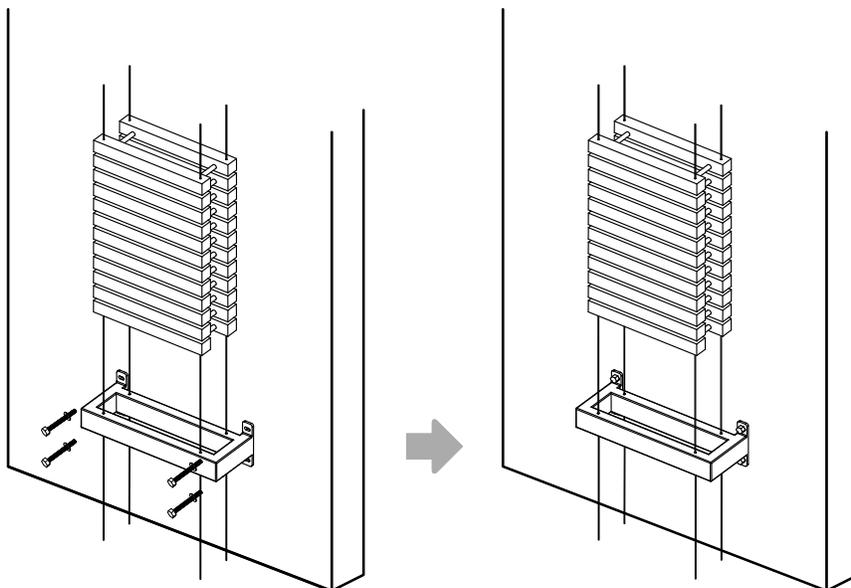
Cut cables below the bottom wall mount. Be sure you do not cut the cable too short. NOTE: Use cable cutter to cut cable.
