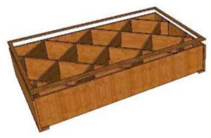
STEP 5. ATTACH (1)  $2\frac{1}{4}$ " x  $63\frac{3}{4}$ " FACE TRIM TO BOTTOM OF BIN, (1)  $1\frac{1}{4}$ " X  $63\frac{3}{4}$ " FACE TRIM TO TOP & (1ea.)  $1\frac{1}{4}$ " X  $36\frac{1}{4}$ " FACE TRIM TO EACH SIDE OF BIN w/ FINISH NAILS. STAND UPRIGHT
