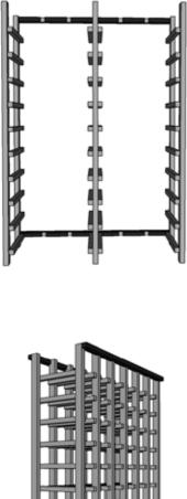
If using rack on top of a base you can nail through the bottom spacer bar of the upper rack into the top spacer bar of an assembled base rack. It is recommended you secure both racks to a wall for optimal stability. Hardware for attaching to a wall is not supplied. Simple "L" brackets from your local hardware store are a popular option for securing to a wall.
