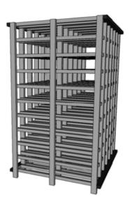
If using rack on top of a base you can nail through the bottom spacer bar of the upper rack into the top spacer bar of an assembled base rack. It is recommended you secure both racks to a wall for optimal stability. Hardware for attaching to a wall is not supplied. Simple "L" brackets from your local hardware store are a popular option for securing to a wall.
