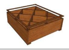
STEP 5. ATTACH (1)  $2\frac{1}{4}$ " x  $36\frac{3}{4}$ " FACE TRIM TO BOTTOM OF BIN, (1)  $1\frac{1}{4}$ " X  $36\frac{3}{4}$ " FACE TRIM TO TOP & (1ea.)  $1\frac{1}{4}$ " X  $36\frac{1}{4}$ " FACE TRIM TO EACH SIDE OF BIN w/ FINISH NAILS. STAND UPRIGHT
