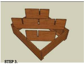
FLIP BIN OVER. SLIDE (2) SHORT SHELVES & (1) LONG SLELF INTO SLOTS AS SHOWN. ENSURE SHELF NOTCHES FACE UP.
