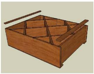
STEP 5. ATTACH (1)  $2\frac{1}{4}$ " x  $32\frac{1}{4}$ " FACE TRIM TO BOTTOM OF BIN. ATTACH (1)  $1\frac{1}{4}$ " X  $32\frac{1}{4}$ " FACE TRIM TO TOP OF BIN w/ FINISH NAILS.
