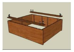
STEP 2. ATTACH (1) LEFT & (1) RIGHT CLEAT w/ SCREWS
