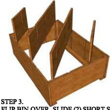
FLIP BIN OVER. SLIDE (2) SHORT SHELVES & (2) LONG SLELF INTO SLOTS AS SHOWN. ENSURE SHELF NOTCHES FACE UP AND ALIGN.
