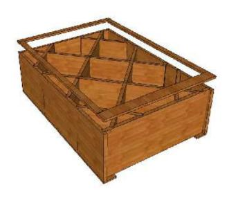
STEP 5. ATTACH (1)  $2\frac{1}{4}$ " x  $27\frac{3}{4}$ " FACE TRIM TO BOTTOM OF BIN, (1)  $1\frac{1}{4}$ " X  $27\frac{3}{4}$ " FACE TRIM TO TOP OF BIN AND (2)  $1\frac{1}{4}$ " X  $36\frac{1}{4}$ " FACE TRIMS TO SIDES w/ FINISH NAILS.
