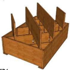
STEP 4. SLIDE (2) SHORT SHELVES & (2) LONG SLELF INTO SLOTS AS SHOWN. ENSURE SHELF NOTCHES FACE DOWN.
