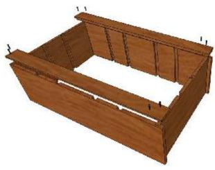
STEP 2. ATTACH LEFT AND RIGHT CLEATS TO BACK OF BIN WITH GLUE AND SCREWS AS SHOWN
