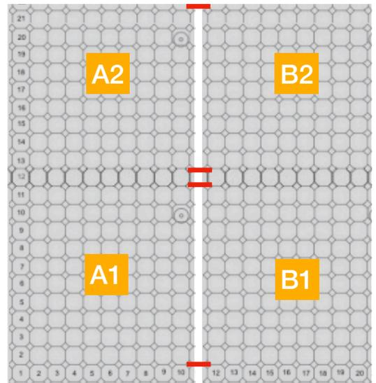
b. Connect A1 to B1, A2 to B2 by inserting the **METAL CONNECTOR PIECES** along the middle column where the **PLASTIC CONNECTOR CLIPS** were inserted in step 3a
