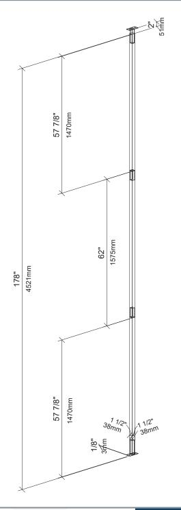
Cut to Fit on Site With Mounting Base extened 2" (51mm), max installation height is 180" (4572mm).
