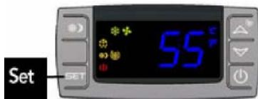
The cooling unit is factory preset with a Minimum Set Point of 58°F and a Temperature Differential of 4°F. This means that the cooling unit will turn on when the display rises above 62°F (58°F + 4°F), and turn off when the display falls below 58°F. In this example, the average temperature inside the cellar will be 60°F.
