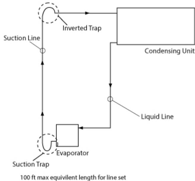
3. **When the evaporator is located above the condensing unit,** pipe suction line with inverted trap as shown to prevent liquid migration to the compressor during the off cycle. The vertical lift of the liquid line is limited to 30 feet. The lift may be increased to 60 feet if an optional liquid/suction Heat Exchanger is added to the field piping.
