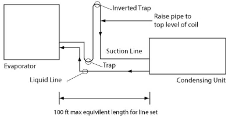
2. **When the evaporator is located below the condensing unit,** a suction trap must be installed at the evaporator, and an inverted trap must be installed at the condensing unit, for proper oil return, as follows:
