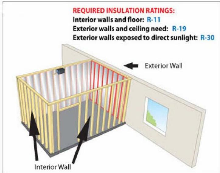
It is important that all walls, joints, doors and windows, electrical outlets and/or switches, pipes, vents and light fixtures be sealed to prevent air and moisture from entering the cellar. If there is a leak in the cellar, the cooling unit will build up excess condensation.
