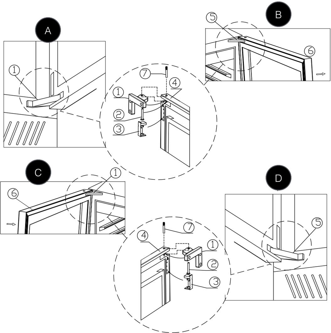
1. As shown in Figure A, use a flat-blade screwdriver to open the upper hinge buckle to see the hinge shaft, and then use a flat-blade screwdriver to pry the hinge shaft and take it out. Then unscrew the lower hinge in the same way.
