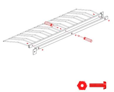
4. **Mount presentation rack to frame** – Align the presentation rack mounting plate with the mounting hole on upright. Using an IDR-PR assembly bolt and washer, insert the bolt through presentation rack and upright, complete with second washer, and nut. Tighten with two 14mm open end wrenches (do not overtighten as this may deform the upright tube). Repeat for the
