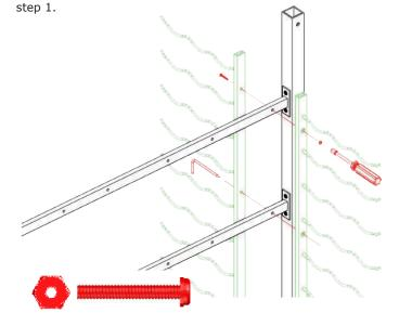
3. **Assemble presentation rack** – Position presentation rack (IDR-PR) piece and presentation rack rail (IDR-H-PRR) back to back as shown. Using the nut driver (included) and a Phillips head screwdriver, fasten the presentation rack and rail together with IDR-PR assembly screws. Fully tighten.
