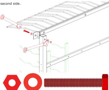
5. **Finishing steps** – Ensure all screws and bolts are fully tightened (especially Crossrail Assembly Screws) and snap mounting hole
